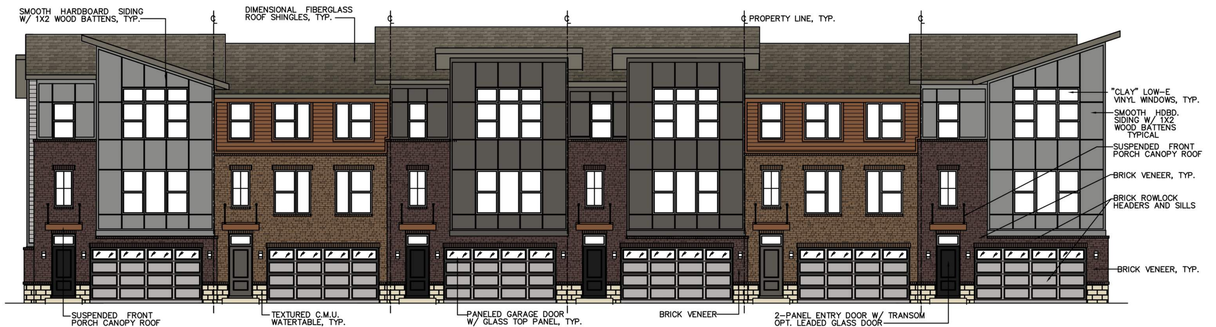
6-UNIT BUILDING FRONT ELEVATION
